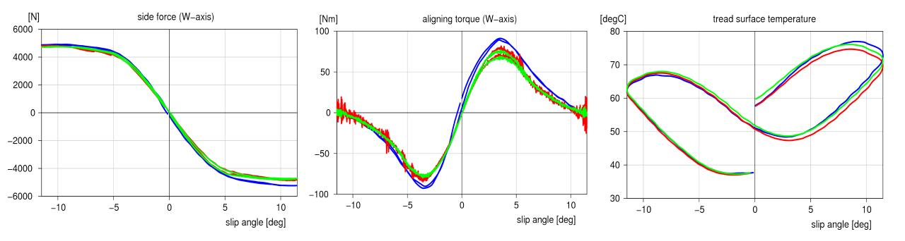
Measurement FTire Real-Time FTire standard
