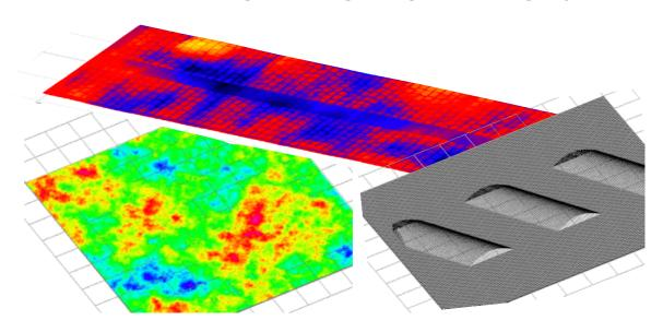
Regular grid based high-resolution 3D road surfaces with curved centerline including location-dependent friction and flexibility properties
